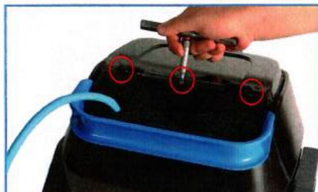
7.1 Use a flat screwdriver to remove the protective grill.
