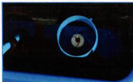
7.4 Check if hair or any foreign object is caught under the impeller. Remove any found.
