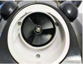
9.3: Snap the flap assembly back after cleaning
