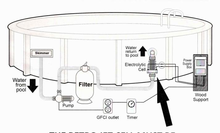
THE RETRO JET CELL MUST BE INSTALLED TO THE RETURN ON THE POOL
