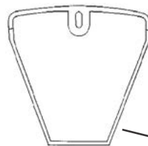
TOP VIEW OF CURVED SIDE ANGLE SUPPORT: Larger than straight side support. Has back wall. Use on curved end uprights. Back wall
