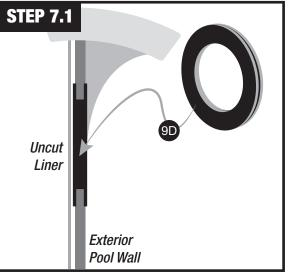
**STEP 7.1** Working from the outside of the pool, install the return fitting double gasket (9D) at the return cutout in the pool wall. For a new pool installation, the inside part of the double gasket would be placed on the metal pool wall, behind the liner. If it's an existing pool, the inside part of the gasket can be placed in either location (behind or on top of the vinyl liner). The outside part of the double gasket always sits against the outside of the metal pool wall.
