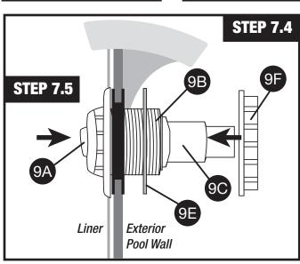
**STEP 7.4** Working from the outside of the pool, screw hose fitting (9C) into return fitting (9B), place plastic washer (9E) onto return fitting threads. Using lock nut (9F) secure washer/return fitting in place by tightening lock nut.
