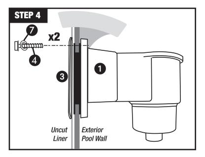
**STEP 4** Push and insert the screws with gaskets (4/7) through the two holes that have been pierced in the liner. Working from outside the pool, align the skimmer body (1) with these screws. Lightly tighten the two screws.
