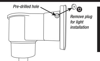
**NOTE:** This skimmer has a predrilled hole for installation for the LED Skimmer Face Plate Light (ACM-197, ACM-197C).
