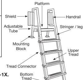
Note: Assemble this ladder before assembling the Confer-Step-1X. If you have already assembled the Confer-Step-1X it will be necessary to remove the handrails (see step #10).
