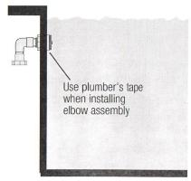
Screw the Elbow Assembly into the return jet using plumber's tape on the threads.
