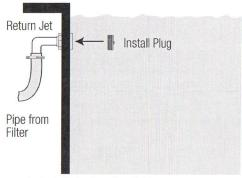
Install plug in return jet to prevent water flow.
