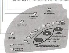
Illuminates when there is no flow or low flow through the Cell. The pool filter pump could be in its "off" cycle. If this is not the case, refer to the Troubleshooting section in this manual.
