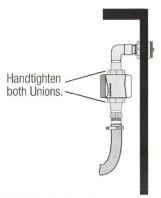
Position the Vessel in a manner where the Cell can be easily inserted and removed. Secure the Vessel by handtightening both Unions.
