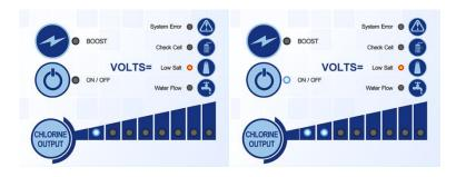
Again you will see alternating lights flashing on the Chlorine Output bar. Each flash represents a number. The example above reads 12 volts. Good range is between 12-14 volts. Anything above 14 indicates low salt, dirty cell or connection problem. The higher the volts means even less salt or an even dirtier cell. Anything less than 12 volts is an indication the salt is too high or there is something stuck in the cell causing a short.
