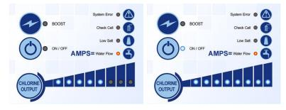
You will see alternating flashing on the system. Each flash of the chlorine output lights represents a number; the example above is reading 5.8 amps. You may see the lights change a little while watching it flash.
