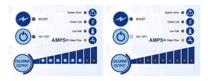
This example would read as 6.0 amps. Readings between 5.8 - 6.0 is the target range if you have 3500ppm salt and the Chlorine Output is set to max. If not in the 5.8 - 6.0 range, Chlorine Output was not set to max or there is low salt in the pool.
