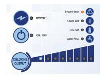
Problem: 1 Chlorine Level Light Lit Cell Cable Disconnected or Very Very Low Salt
