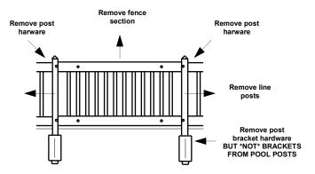
Step 3 Remove the post hardware used to secure section in place (both sides of section). Keep this hardware & remember positioning as you will require it to reassemble. Remove fence section & remove the two line posts. Keep all hardware for reassembly. Note: you may have some extra hardware left over once complete as line posts have double for opposite sections. DO NOT REMOVE MOUNTING BRACKETS FROM POOL UPRIGHT POSTS
