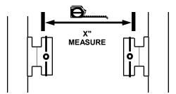
Step 5 Measure distance from inside of bracket to inside of bracket from the left end post to the right end post. Mark this length/measurement on the fence section. Make certain to balance distance from each end picket on both ends of section so final installation looks neat & balanced. Cut rail ends accordingly
