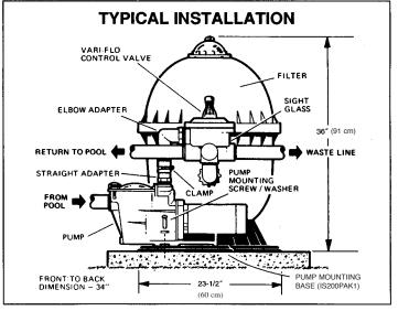
NOTE: If rigid return piping is used, installation of a piping union is recommended for ease of future servicing.
